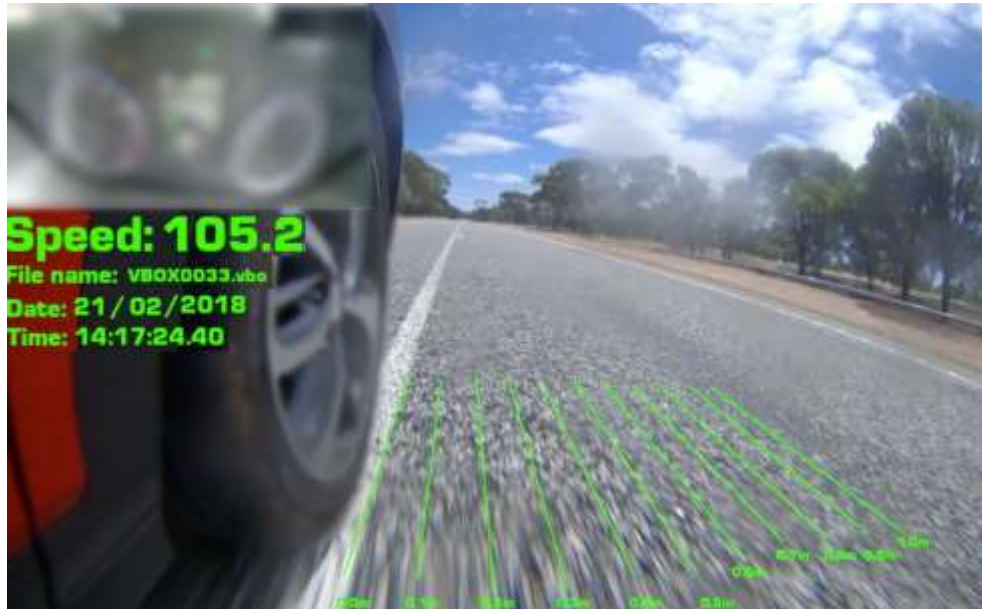
Figure 2.1 Camera layout used to record line crossing events
