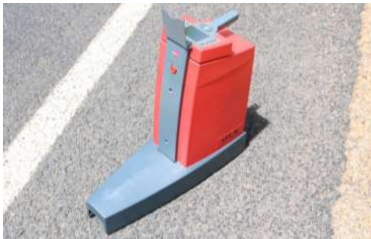
Figure 2.3 The LTL-X Retroreflectometer
