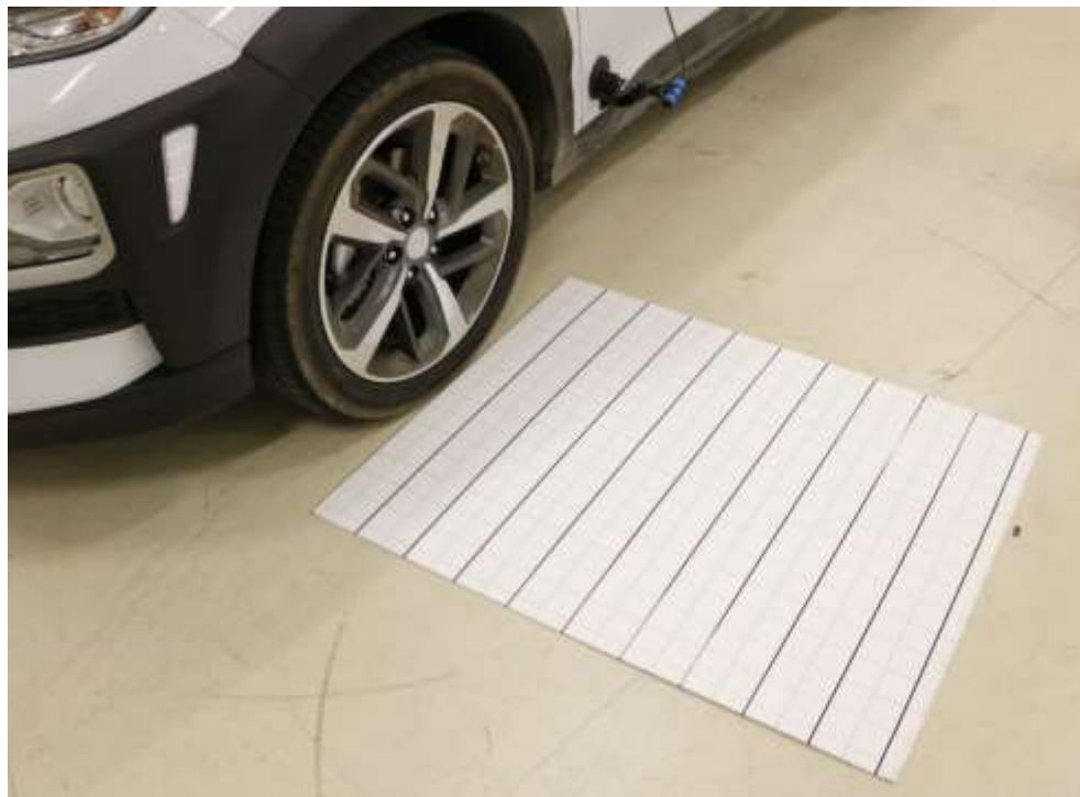
Figure 2.2 Camera overlay being aligned using scale
